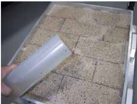
Figure 4. Supplying water to blocks
